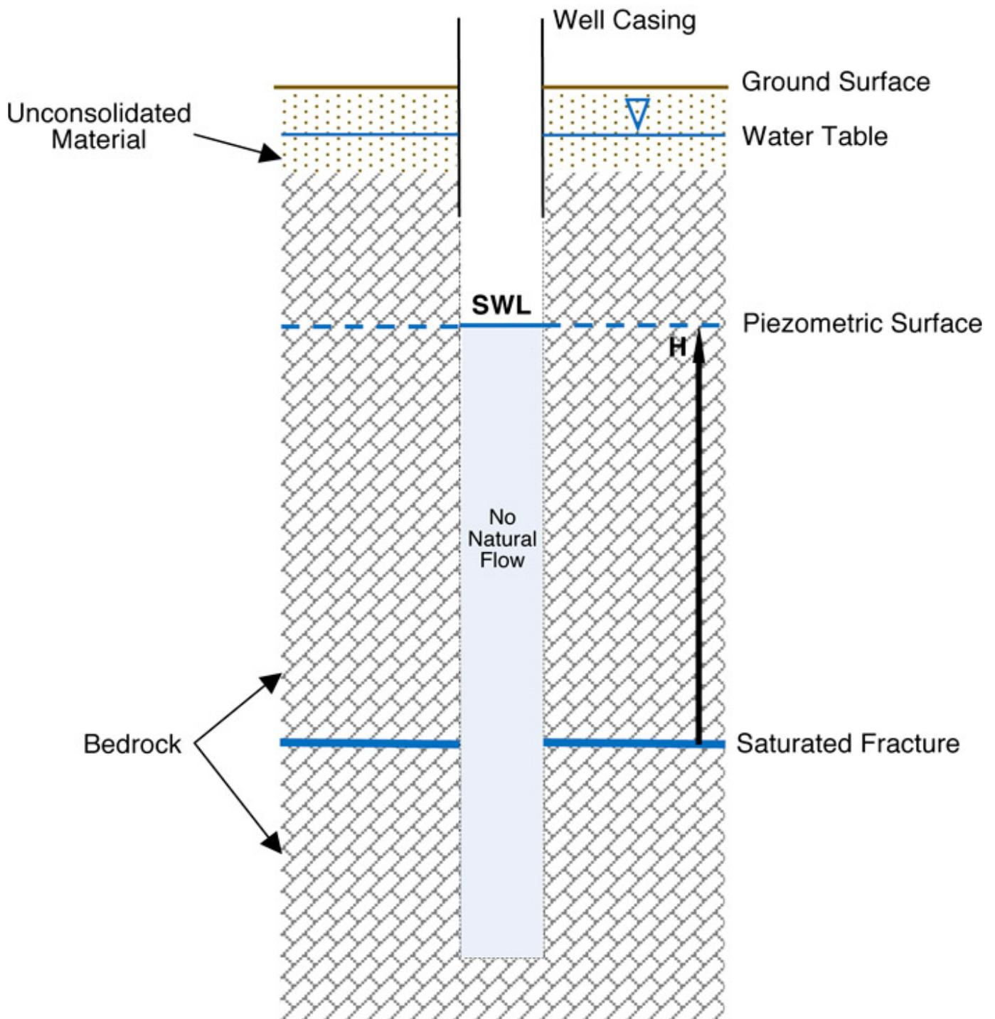
**Figure 3-8. Open borehole piercing one confined fracture, no natural borehole flow (Not to Scale) H = Head; SWL = Static Water level**
