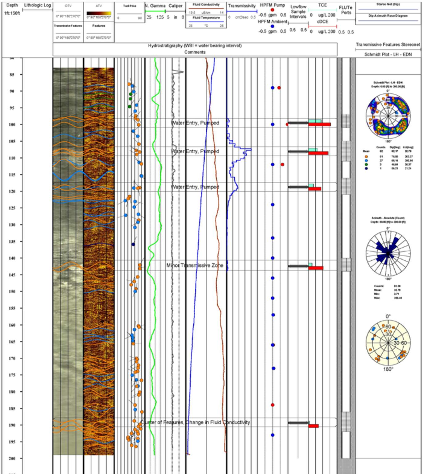
**Figure 5-4. An example of an integrated borehole log.**
