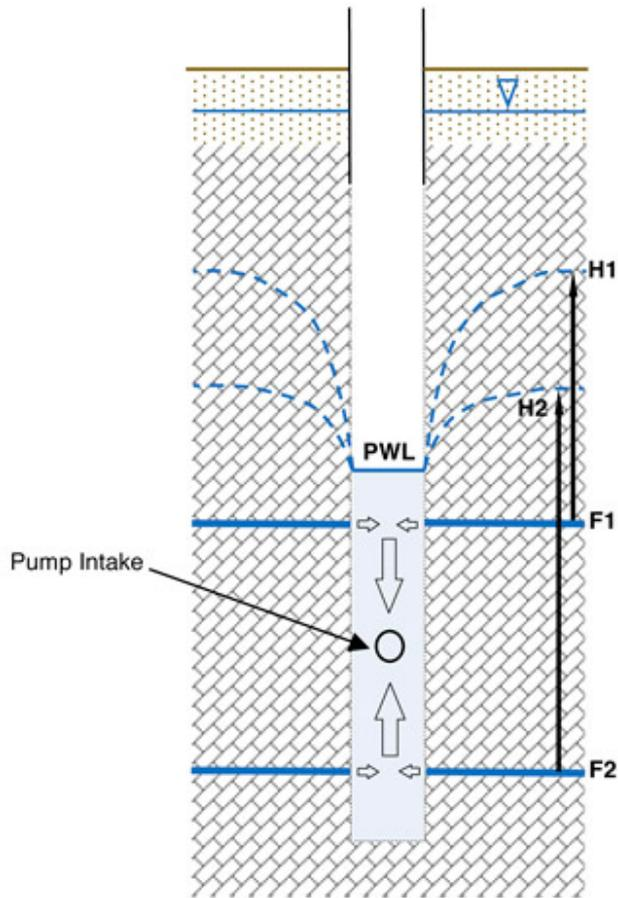
**Figure 3-11. Open borehole two confined fractures pumping condition (not to scale)**
