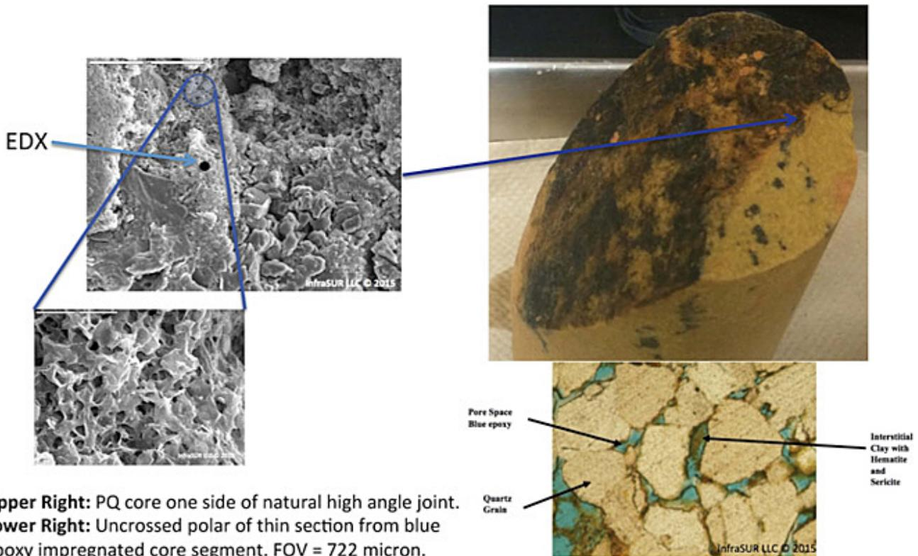
**Upper Right:** PQ core one side of natural high angle joint.
