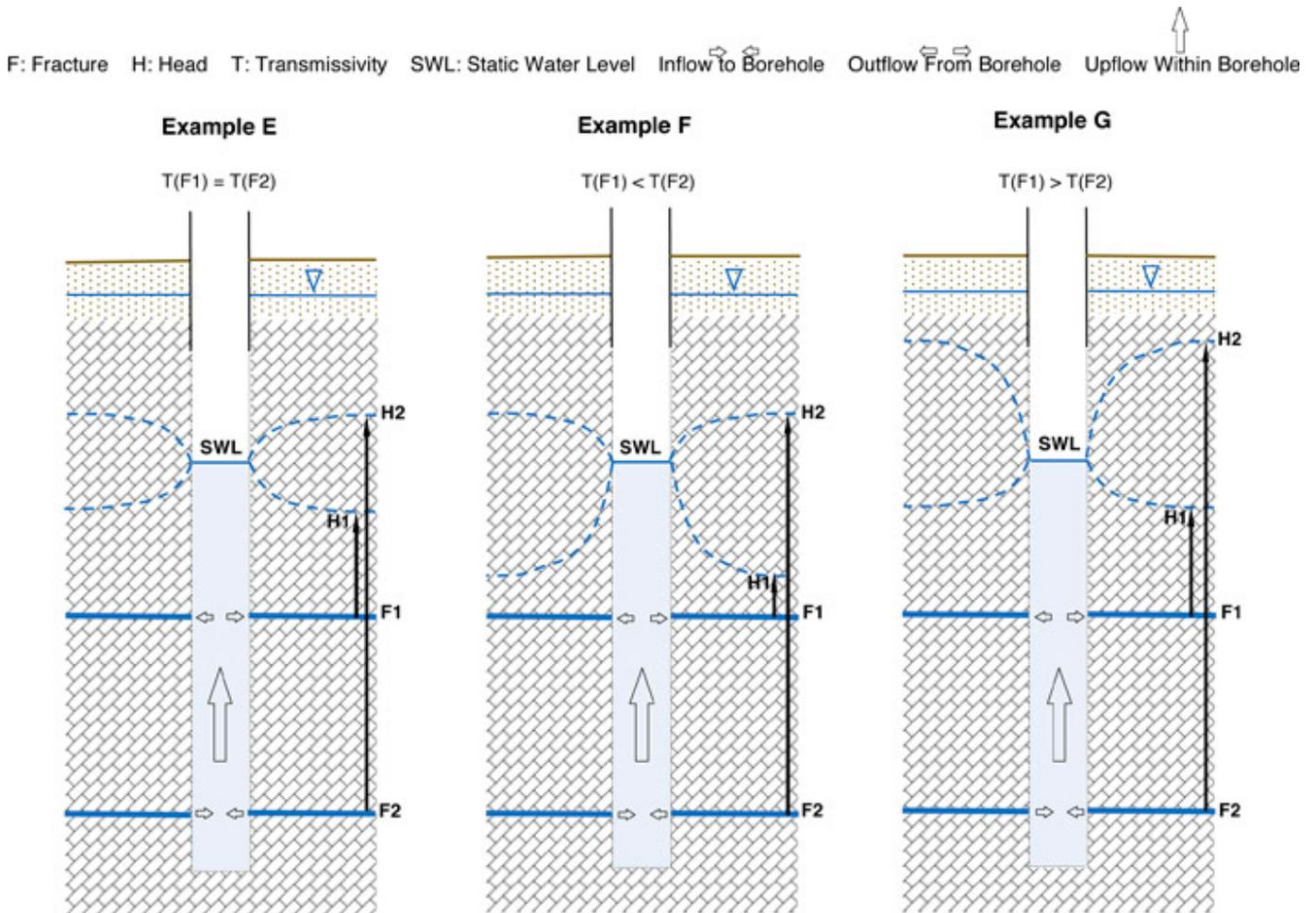
**Figure 3-10. Open borehole piercing two confined fractures, natural borehole up flow.**
