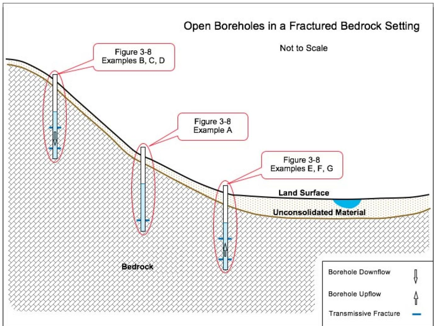
**Figure 3-7. Open boreholes in a fractured rock setting.**
