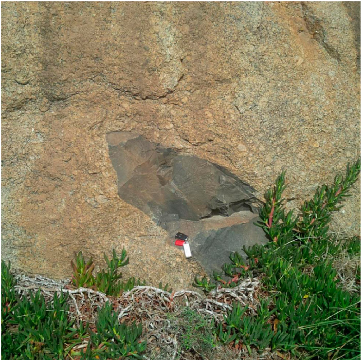
Figure B-3. Aphanitic, mafic intrusion into phaneritic pluton (granite); note thermal aureole in country rock (pink/orange discoloration surrounding mafic intrusion). Thermal aureole is susceptible to differential weathering and permeability.
